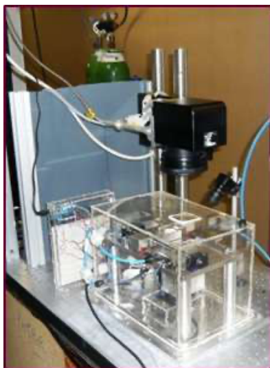
Figure 8.7: Example additive manufacturing platform that can fit within the experimental facilities, the 'shoe box' laser additive manufacturing system which was used by Bidare et al. in monitoring the process using high-speed imaging
