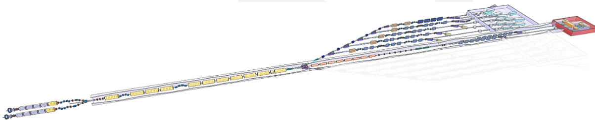
Figure 7.5: Phase 1c, representing the 'nominal' configuration based on 6 FELs supplying up to 18 end stations.
