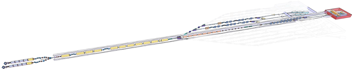
Figure 7.4: Phase 1b, including dual photoinjector, normal conducting booster, and MEC hall including beamlines and laser infrastructure.
