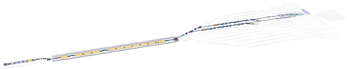
Figure 7.3: Phase 1a, consisting of a 8 GeV superconducting linac driven by a single photoinjector, and 2 FEL beamlines (SXR/HXR).
